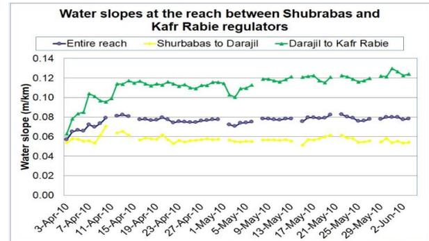
Figure 6. water slopes for different reaches between Shubrabas and Kafr Rabie cross regulators
