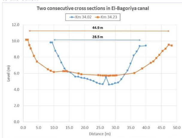
**Figure 9. Two consecutive cross-sections in El-Bagoriya with different widths**
