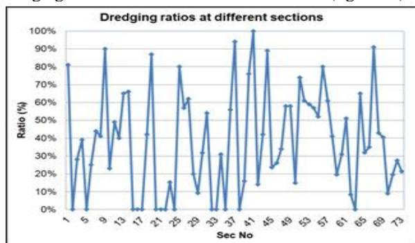
**Figure 14. Dredging ratios at different sections**
