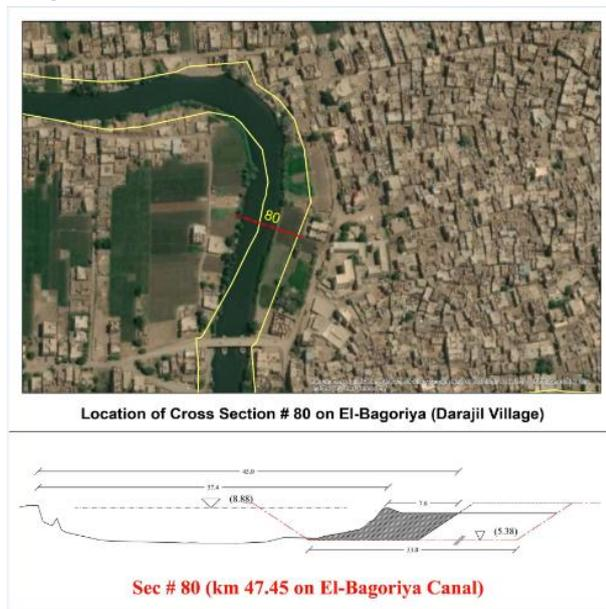
**Figure 11. Adapting the required dredging in sec # 80 (Km 47.45)**
