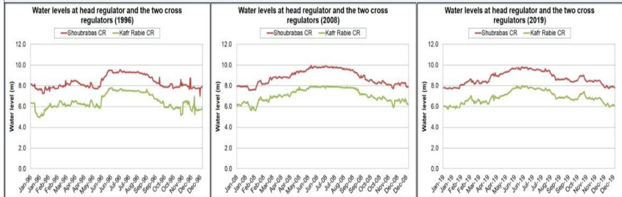
Figure 5. daily water levels downstream the head regulator, downstream Shubrabas regulator and upstream Kafr Rabie cross regulator
