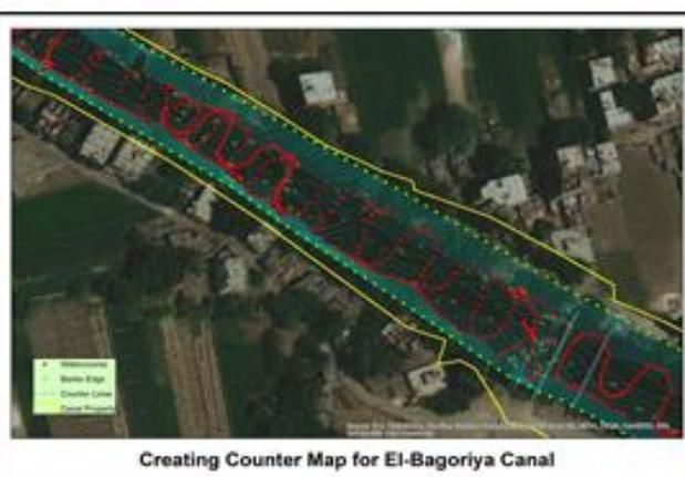
**Figure 8. Surveyed points and the developed counter map for El-Bagoriya watercourse**
