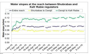
Figure 6. water slopes for different reaches between Shubrabas and Kafr Rabie cross regulators
