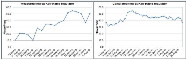
Figure 4. Daily water supply values downstream the head regulator and downstream Kafr Rabie cross regulator during three different years
