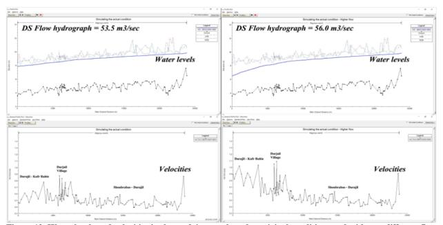
Figure 12. Water levels and velocities in the studying reach under original conditions and with two different flow values
