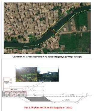
Figure 10. Adapting the required dredging in sec # 70
