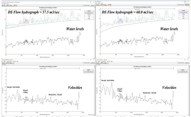
Figure 15. Water levels and velocities in the studying reach for post-dredging situation and with two different flow values
