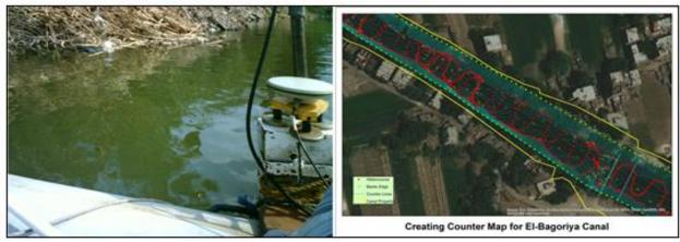
Figure 8. Surveyed points and the developed counter map for El-Bagoriya watercourse
