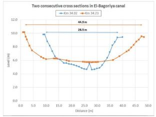
Figure 9. Two consecutive cross-sections in El-Bagoriya with different widths
