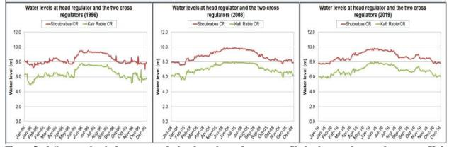
Figure 5. daily water levels downstream the head regulator, downstream Shubrabas regulator and upstream Kafr Rabie cross regulator
