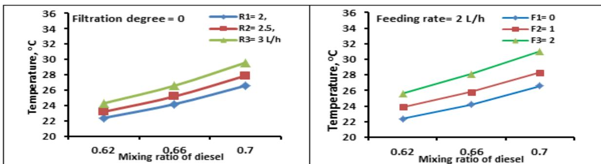
Fig.6. The effect of the mixing ratios on the temperature of mixing diesel to (UEO).
