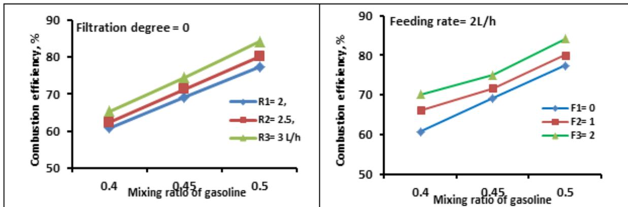
**Fig.7. The effect of the mixing ratios on the combustion efficiency of mixing gasoline to (UEO).**
