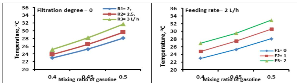
Fig.5. The effect of the mixing ratios on the temperature of mixing gasoline to (UEO).
