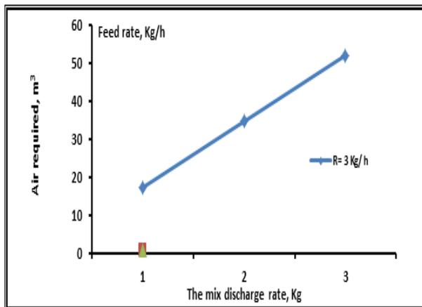
**Fig. 1. The quantity of air required for the disposal of different rates mixture of (UEO) each of diesel and gasoline to determine the air pump speed**
