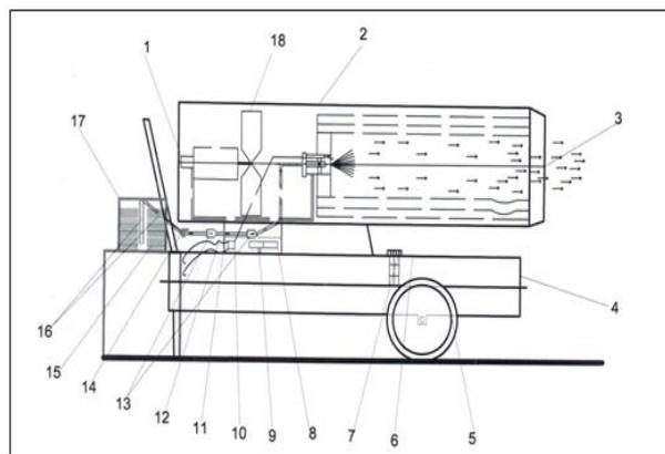
Fig .4. The burner model BGO- 30 A after modification
