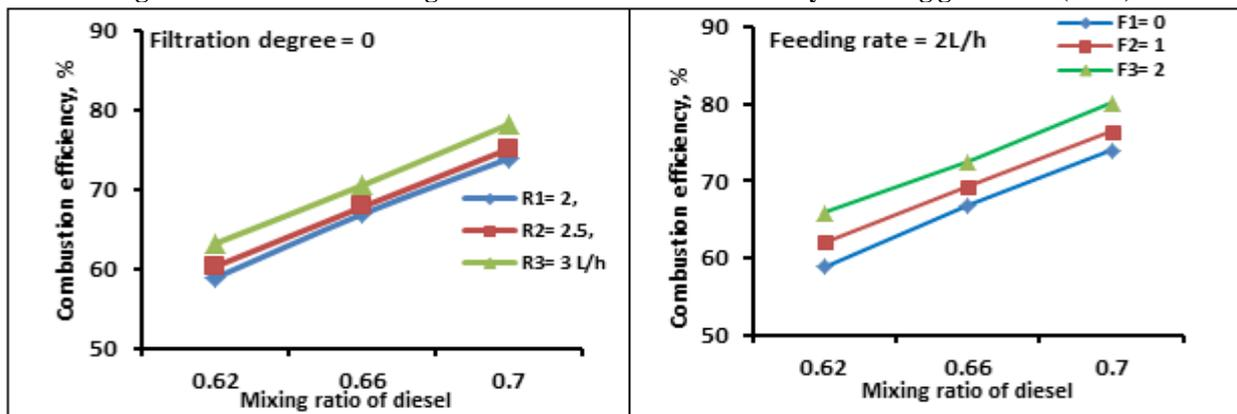
**Fig.8. The effect of the mixing ratios on the combustion efficiency of mixing diesel to (UEO).**
