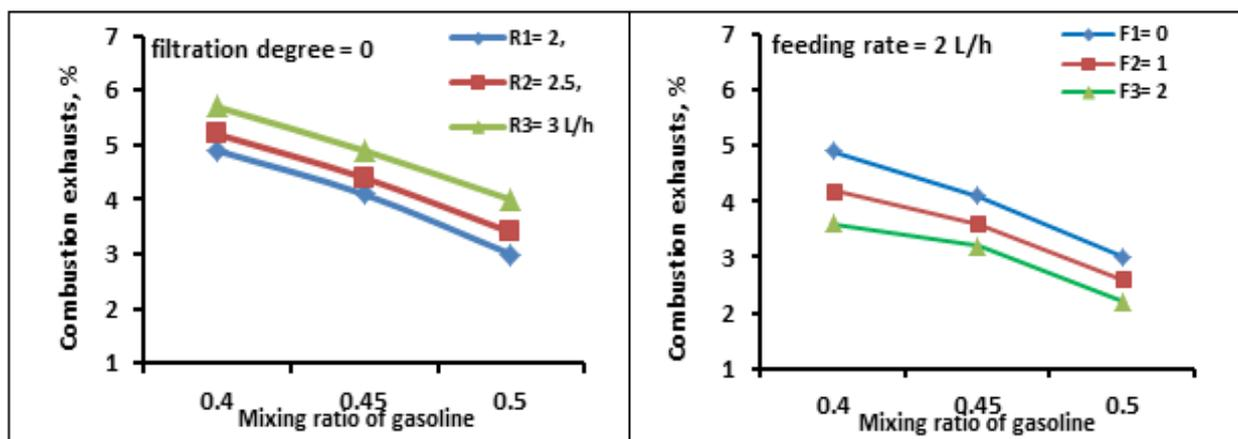
**Fig.9. The effect of the mixing ratios on the combustion exhausts of mixing gasoline to (UEO).**
