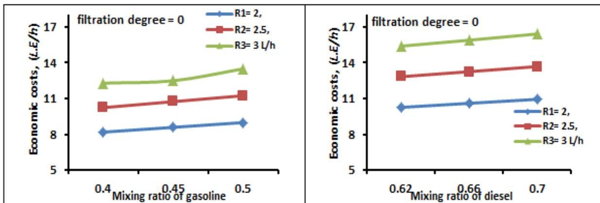
**Fig.11. The effect of the mixing ratios on the economic costs of mixing gasoline or diesel to (UEO).**
