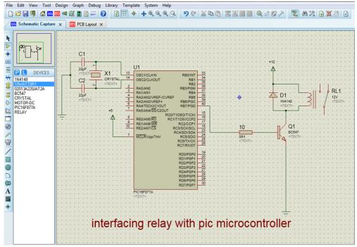
Fig. 4. interfacing relaywith pic microcontroller
