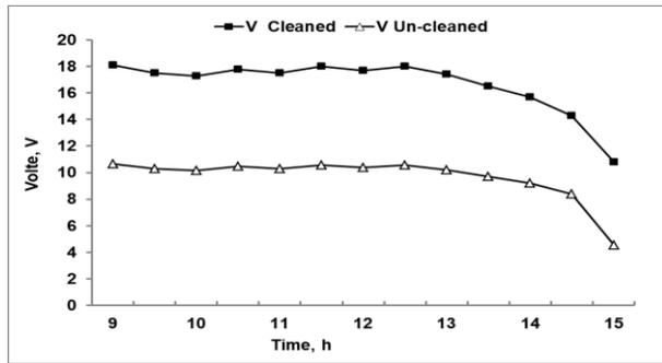
Fig. 6. Variation of voltage for the cleaned and un-cleaned surfaces at the end of dust deposition period (168 days).
