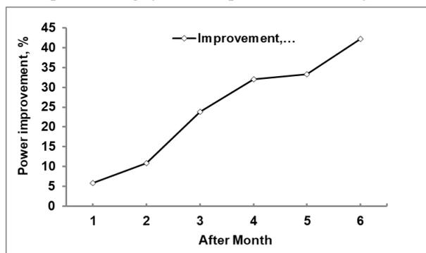
Fig. 9. Variation of power improvement for the cleaned and un-cleaned solar panels.
