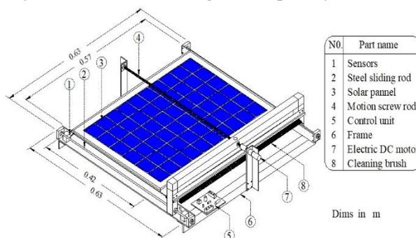
Fig. 1. Solar panel cleaning system
