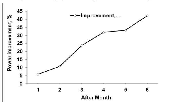
Fig. 9. Variation of power improvement for the cleaned and un-cleaned solar panels.
