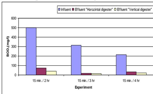
Fig. 10. BOD values at 40 °C digestion temperatures with stirring time of (15 min. / 2 hr, 15 min. / 3 hr and 15 min. / 4 hr).
