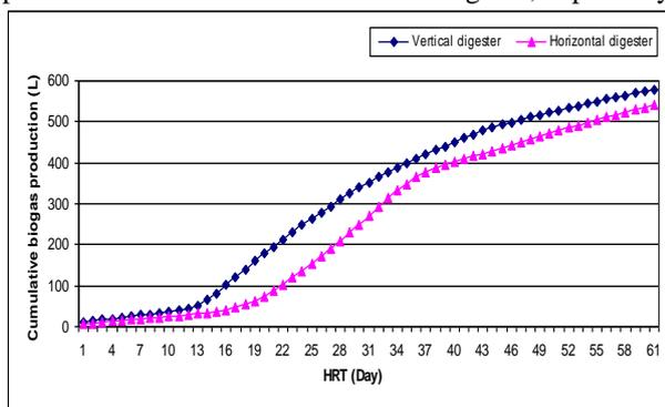
**Fig. 5. The cumulative biogas production from the two biogas digesters at 40 °C digestion temperature and stirring time of 15 min. / 3 hr.**
