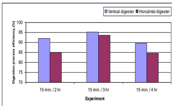
**Fig. 12. Digestion process efficiency at 40 °C digestion temperatures with stirring time of (15 min. / 2 hr, 15 min. / 3 hr and 15 min. / 4 hr).**
