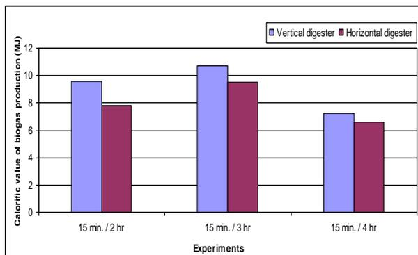
Fig. 8. Calorific value of biogas production at 40 °C digestion temperatures with stirring time of (15 min. / 2 hr, 15 min. / 3 hr and 15 min. / 4 hr).
