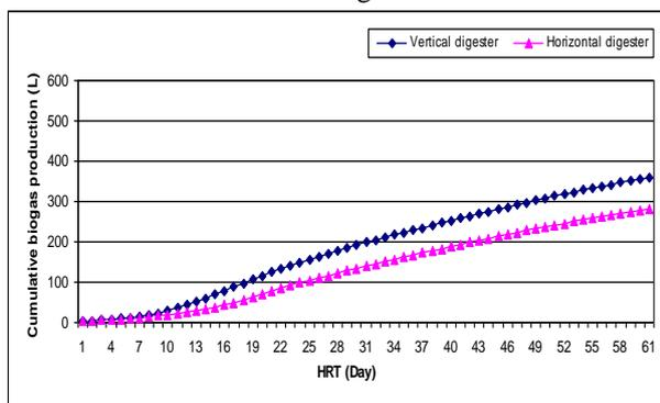
**Fig. 2. The cumulative biogas production from the two biogas digesters at 35 °C digestion temperature and stirring time of 15 min. / 2 hr.**
