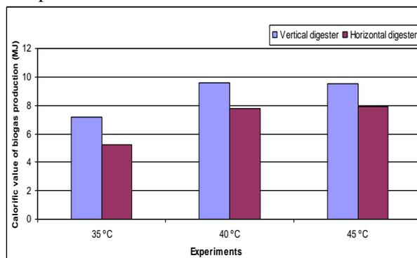
**Fig. 7. Calorific value of biogas production at (35 °C, 40 °C and 45 °C) digestion temperatures and stirring time of 15 min. / 2 hr.**
