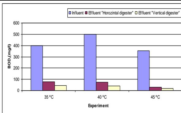
Fig. 9. BOD values at (35 °C, 40 °C and 45 °C) digestion temperatures and stirring time of 15 min. / 2 hr.
