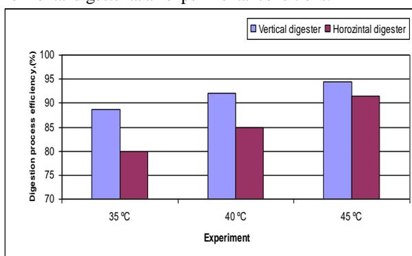
**Fig. 11. Digestion process efficiency at (35 °C, 40 °C and 45 °C) digestion temperatures and stirring time of 15 min. / 2 hr.**
