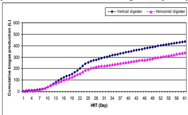
**Fig. 6. The cumulative biogas production from the two biogas digesters at 40 °C digestion temperature and stirring time of 15 min. / 4 hr.**
