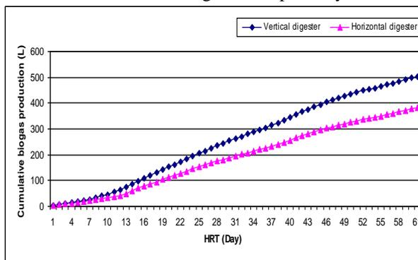
**Fig. 3. The cumulative biogas production from the two biogas digesters at 40 °C digestion temperature and stirring time of 15 min. / 2 hr.**
