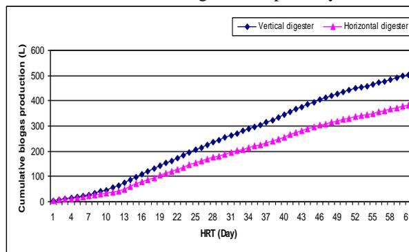
**Fig. 3. The cumulative biogas production from the two biogas digesters at 40 °C digestion temperature and stirring time of 15 min. / 2 hr.**
