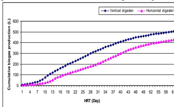
**Fig. 4. The cumulative biogas production from the two biogas digesters at 45 °C digestion temperature and stirring time of 15 min. / 2 hr.**
