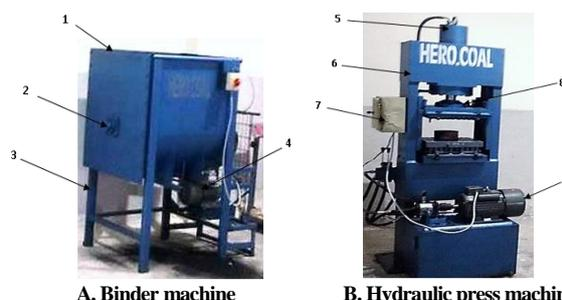
**Fig. 1. The used hydraulic press machine and binder**
