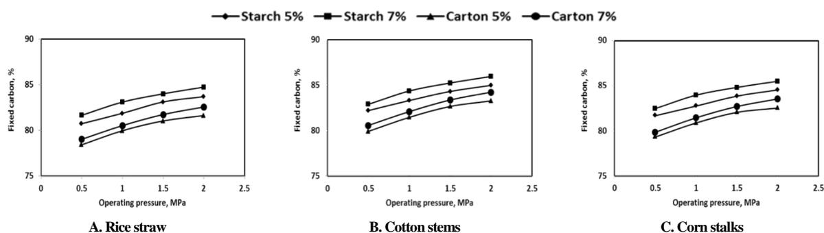
**Fig. 6. Fixed carbon of produced charcoal briquettes at blending materials under different operating pressures**
