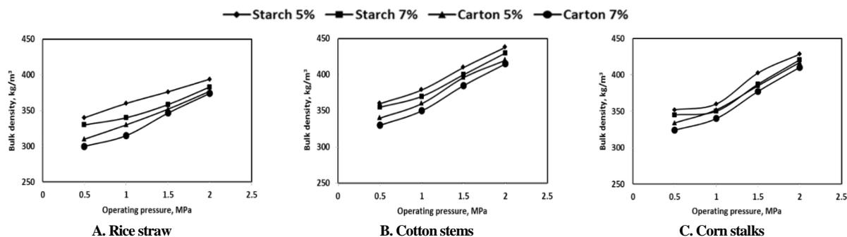
Fig. 4. Bulk density of charcoal briquettes with different blending materials and concentrations under different pressures
