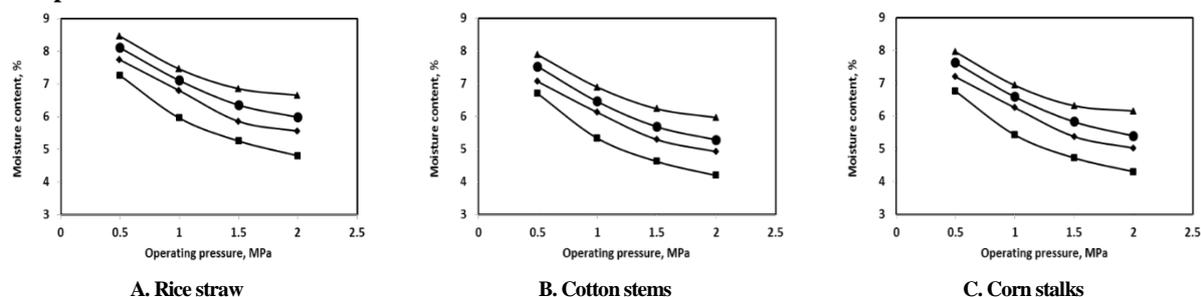
Fig. 5. Briquettes moisture content at different operating pressures
