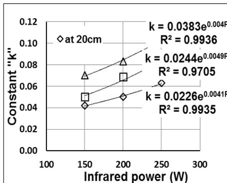
Fig.3.Relationship between constant "k" and infrared power level at different exposure distance.
