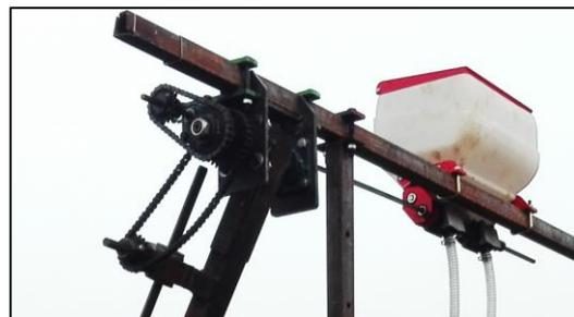
Fig. 5. Transmission components during manufacturing
