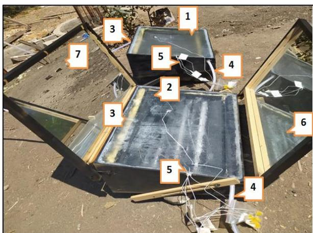
1- Conventional SSS without mirrors 2- Modified SSS with booster mirrors 3-Inlet of saline water 4- Outlet of distillate water
