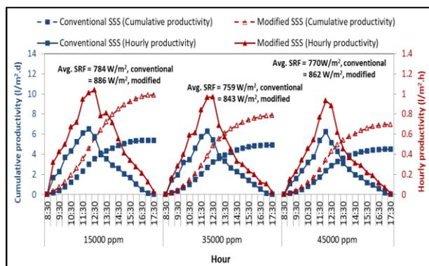
**Fig. 6. Variations of hourly and cumulative distillate water productivity for both conventional and modified SSSs at different salinity levels.**
