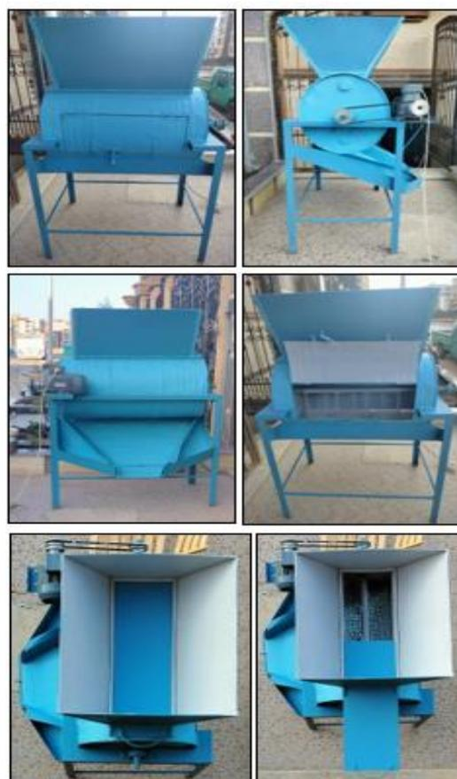
**Fig. 1. Some photos of the developed maize shelling machine.**
