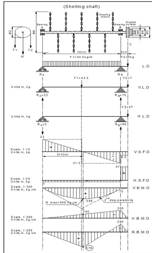
Fig. 4. Stress analysis on shelling shaft.
