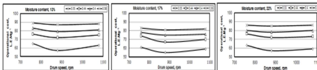
Fig. 9. Some operating parameters affecting on operational cost.
