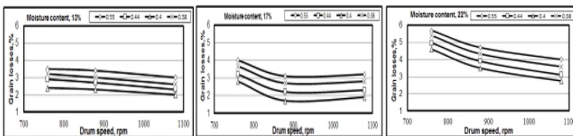
**Fig. 7. Some operating parameters affecting on grain losses.**
