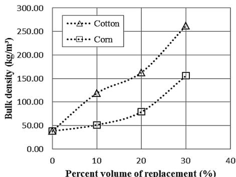
Fig. (3): Effect of material percentage on bulk density at for (TS and CS).
