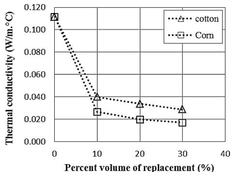
Fig (4): Effect of material percentage on thermal conductivity for (TS and CS).
