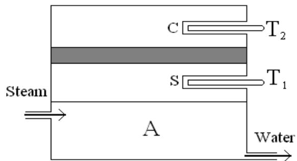
**Fig. 1. A schematic diagram for steam unit and specimen of thermal conductivity Apparatus (C,S) Brass disks, (B) Specimen, (T<sub>1</sub>, T<sub>2</sub>) Thermometers, ElBessoumy,2005).**
