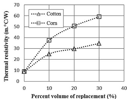
Fig. (5): Effect of material percentage on the intrinsic thermal resistivity for (TS and CS).
