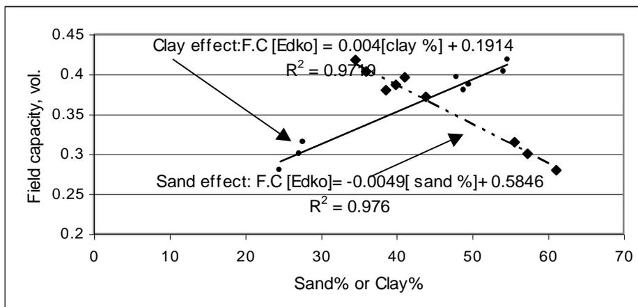
**Fig.6. Correlation between sand and clay contents and estimated field capacity of Edko soil**
