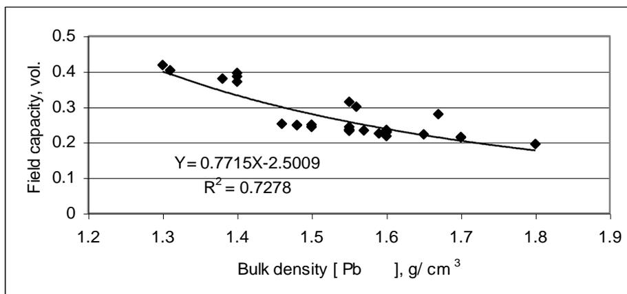
**Fig. 7. General trand of soil bulk density effect on field capacity- all samples from all soils**
