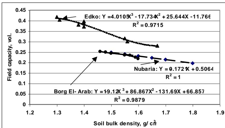
**Fig.4. Correlations between soil bulk density and field capacity for Nubaria, Borg El- Arab and Edko soils**
