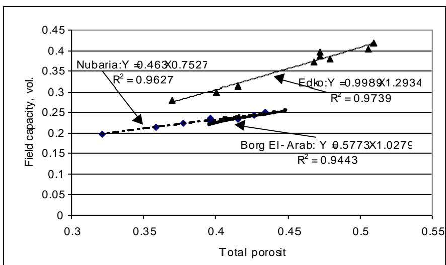
**Fig.5. Correlations between total porosity and field capacity for Nubaria, Borg El- Arab and Edko soils**
