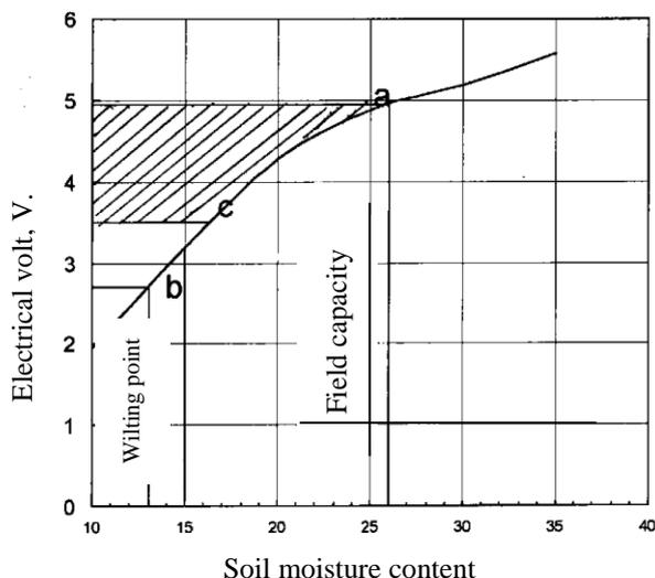
**Fig. 7-B: Calibration of the two-electrode sensors.**
