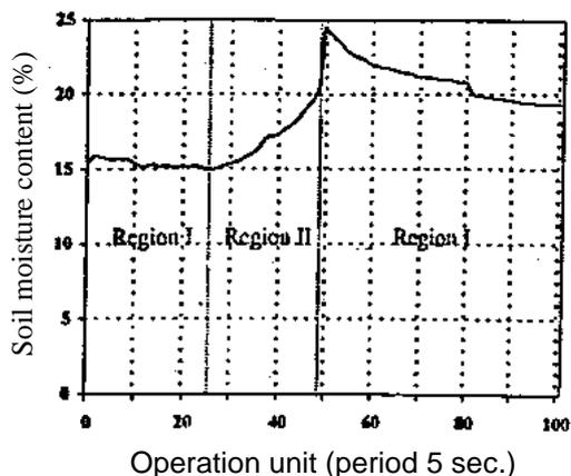
**Fig. (10): Moisture response transient using ON-OFF controller.**
