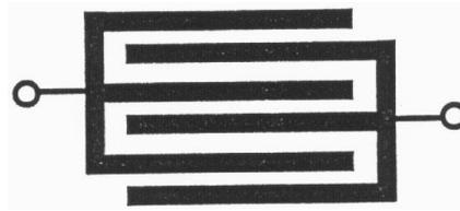
**Fig. 2: The “ E” sensor of soil moisture content.**
