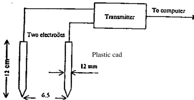
Fig. 3: The two-electrode sensor.
