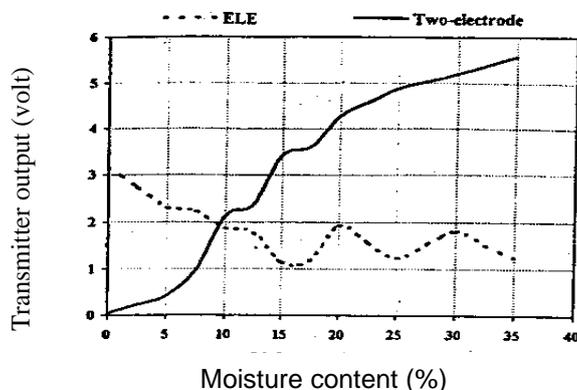
**Fig. (8): Soil moisture content via transmitter voltage.**
