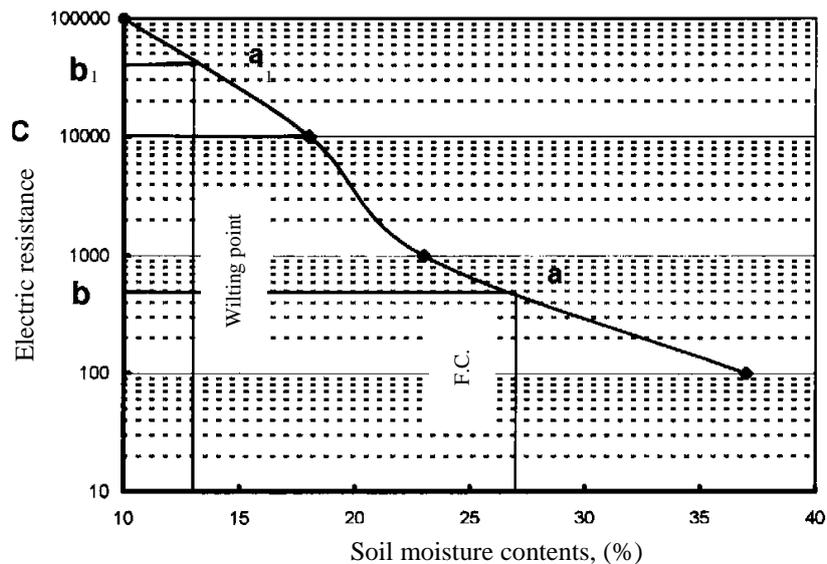
**Fig. 7-a: Calibration of the ELE sensors.**
