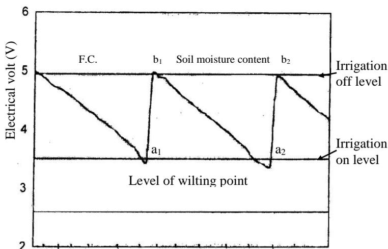
**Fig. (11): The inclination of moisture response of two-electrode sensor.**
