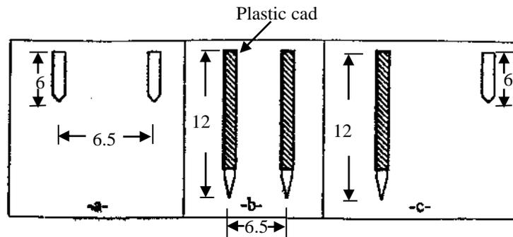
Fig. 4: Different shapes and arrangements of the two-electrode sensor.
