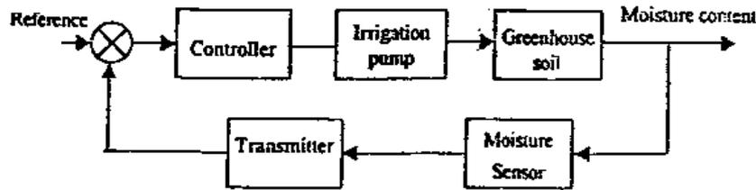
Fig. (6): ON-OFF soil moisture content control block diagram.
