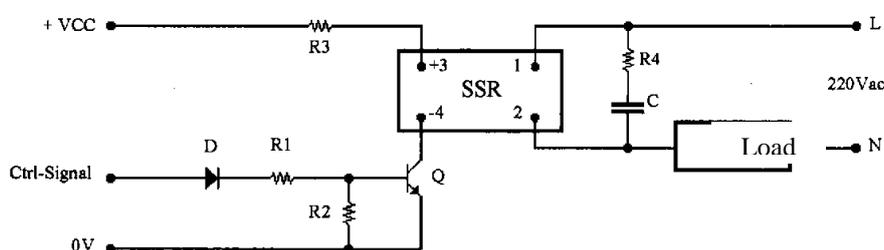
Fig 1: The solid-state relays (SSR) circuit diagram.
