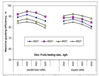
Fig. 4. Machine grading efficiency as affected by different sieve rotating speeds, different fruits feeding rates for both types of sieve cells using okra fruits.
