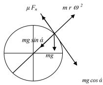
Fig. 2. Forces acting on a particle of fruit in a rotating cylinder
