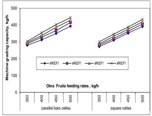
Fig. 3. Machine grading capacity as affected by different sieve rotating speeds, different fruits feeding rates for both types of sieve cells using okra fruits.
