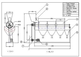
Fig. 1-B. Side view and elevation view of a simple grading machine
