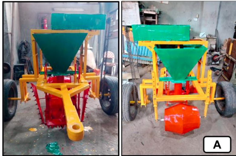
Fig. 2A. Hoeing unit during field experiments
