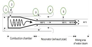
1-adjustable direct fuel injection 2-carburetor with diaphragm air intake valve 3- double cooling jacket 4- cooling air intake and 5- water-injection for pre-cooling
