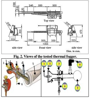
1-air intake 2- carburetor with diaphragm air 3- fuel adjustable screw 4- spark plug 5- combustion chamber 6- fuel intake.
