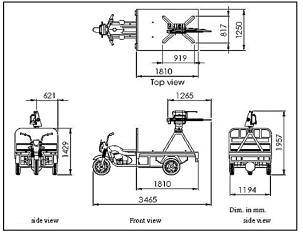
Fig. 5. Views of the tricycle with the tested fogger. Methods
