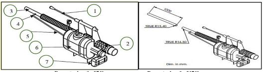
Resonator length of 740 mm 1- hand pump 2- cooling jacket for combustion chamber 3- resonator, 4- shut-off valve 5- chemical flow tube 6- chemical tank 7- fuel tank. Fig. 1. Isometric of the tested thermal fogger.
