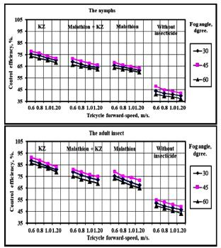
Fig. 6. Effect of tricycle forward-speed, control material, fog angle on control efficiency under resonator length of 74 cm for the nymphs and the adult insect.
