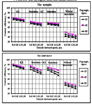
Fig. 7. Effect of tricycle forward-speed, control material, fog angle on control efficiency under resonator length of 174 cm for the nymphs and the adult insect.
