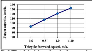
Fig. 8. Effect of tricycle forward-speed on fogger capacity.
