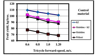
Fig. 9. Effect of tricycle forward-speed and insecticidematerials on "Zaghloul" date palm fruit yield at optimum fog angle of 45° and resonator length of 174 cm.
