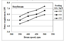
Fig. 10. The required power for threshing operation of soybean
