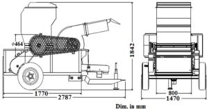
Fig. 2. The outline dimensions of the manufactured thresher
