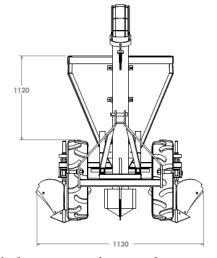
Fig. 1. Schematic diagram of main components for a single-row automatic potato planter
