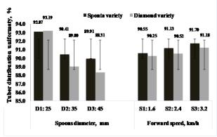
Fig. 5. The tubers distribution uniformity, % as affected by spoons diameter, forward speeds and varieties.
