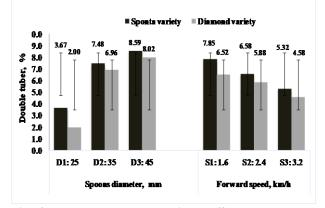
Fig. 4. The double tubers ratio as affected by spoons diameter, forward speeds and varieties.
