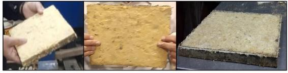
Fig. 4. Manufactured particle boards
