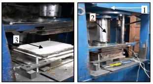
1-main frame, 2-piston, 3- particle board under the manufacturing Fig. 1. The hydraulic press during manufacture particle boards
