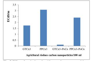
Fig. 5. Effect of agricultural residues carbon nanoparticles on electrical conductivity of tannery effluent
