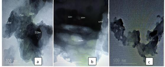
Fig. 1. TEM images of (a) green tea(GTCn), (b)pomegranate peel(PPCn) and (c)potato peels carbon nanoparticles.
