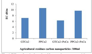
Fig. 4. Effect of agricultural residues carbon nanoparticles on electrical conductivity of tannery effluent
