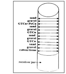
Fig. 2. A pictorial view of installing a salinity treatment filter from tanneries' industrial effluent
