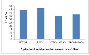
Fig. 3. Effect of agricultural residues carbon nanoparticles on electrical conductivity of tannery effluent
