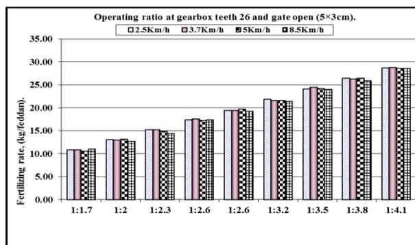
Figure 6. Fertilizing rate according to operating ratio and fast forward speed at gate open (15cm2).
