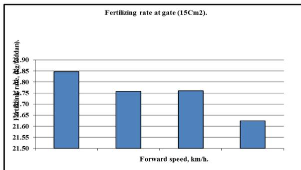
Figure 3. Fertilizing rate according to forward speed
