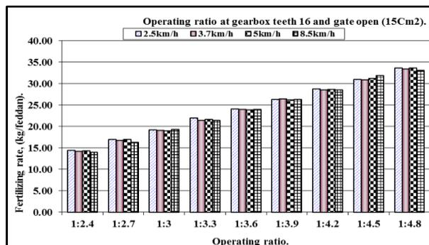
Figure 5. Fertilizing rate according to operating ratio and slow forward speed at gate open (15Cm2).
