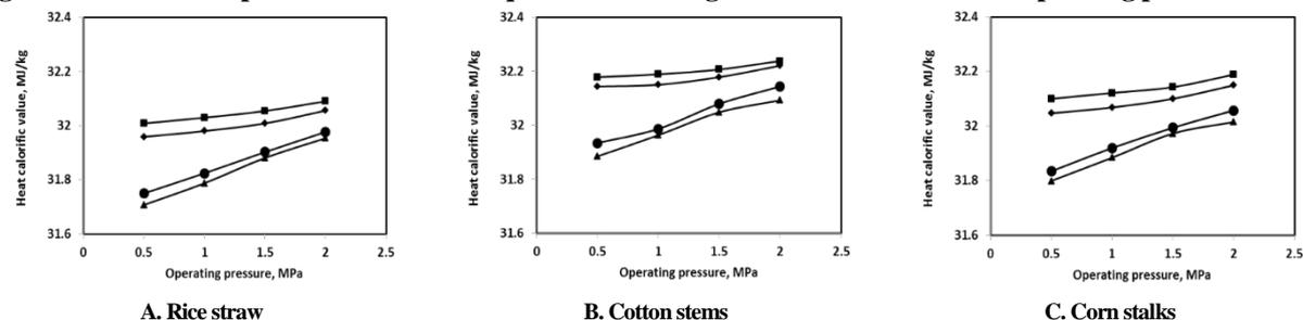
**Fig. 7. Effect of different operating pressures at blending materials on heating calorific value of charcoal briquettes**
