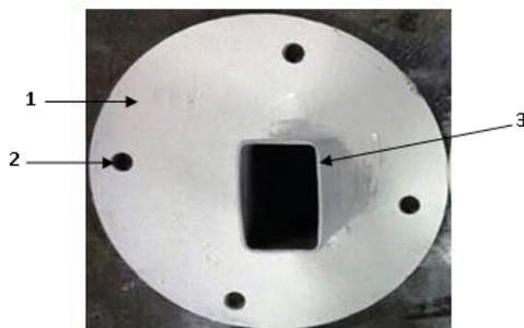
1. Circular Plate frame, 2. Plate hole and 3. Parallel rectangle shape
