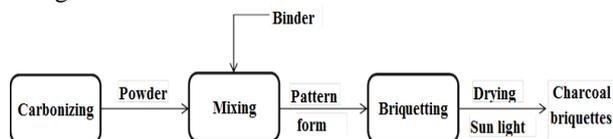
**Fig. 3. Schematic of charcoal briquetting process**
