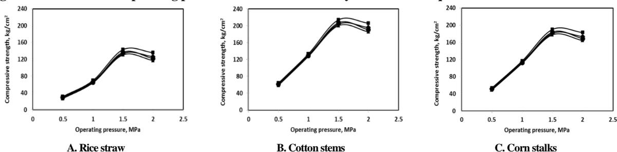
Fig. 9. Compressive strength for charcoal briquettes blending at binder materials and concentrations under different pressures
