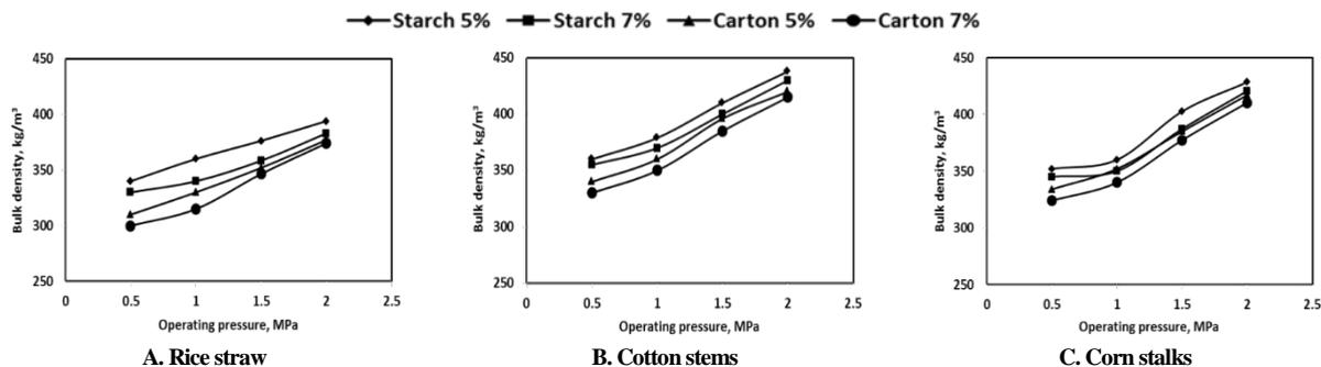
Fig. 4. Bulk density of charcoal briquettes with different blending materials and concentrations under different pressures
