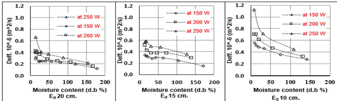
**Fig. 5.** Variation in effective moisture diffusivity "Deff" with moisture content at various infrared power and various exposure distance "Ed" at air velocity 1.5 m/s.
