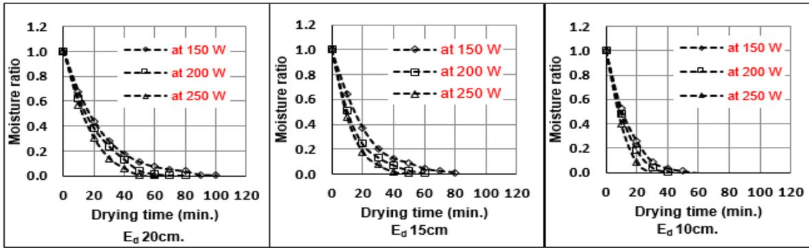
Fig. 2.Effect of Infrared power levels and exposure distances "Ed" on moisture ratio at air velocity 1.5 m/s.
