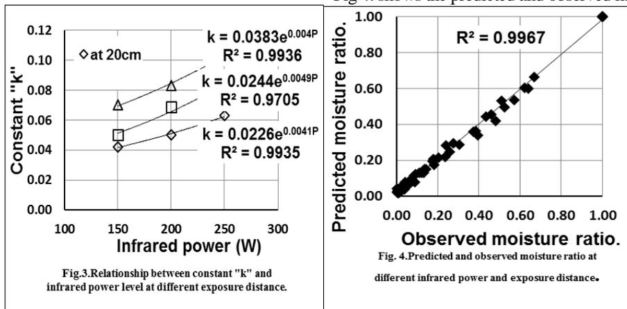
Fig.3.Relationship between constant "k" and infrared power level at different exposure distance.
