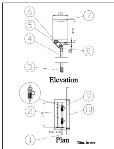
(1) Metering unit input shaft; (2) Agitator ; (3) Steel spring ; (4) Delivery tube; (5) Chain ; (6) Sprocket ; (7) Tank cover; (8) Idler; (9) Rotary distributor (10) Horizontal chassis.
