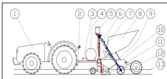
(1)Narrow tires tractor ;(2)Hitch point ;(3)Spraying pump ;(4)Liqued stralization chemical tank ;(5)Nano fertilizer tank ;(6)Main Chsises ;(7)Telescopic arm;(8)Tubers tank;(9)Tipping tuber tank hydraulic cylinder;(10)planting opener;(11)Planted tubers covering discs;(12) Planter rear wheel;(13) potato rows.
