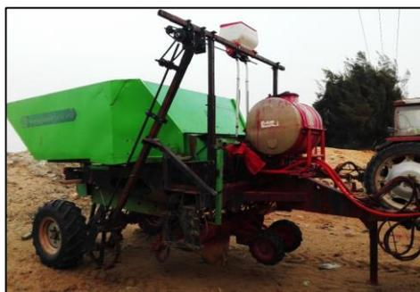
**Fig. 9. Assembling the nano fertilizer metering unit on the potato planter**
