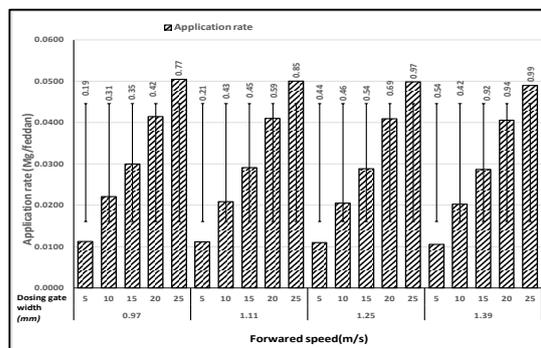
**Fig. 10. Effect of metering gate width at different planting forward speeds on fertilizer application rate**
