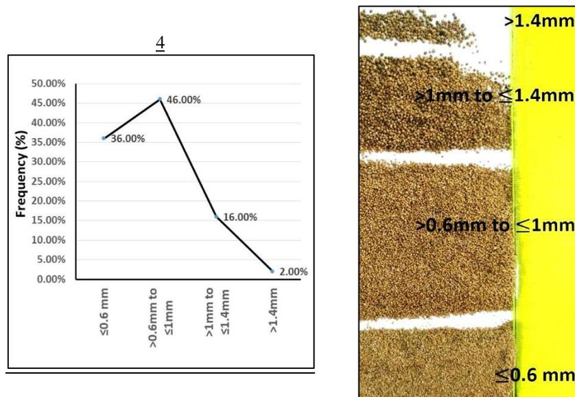
(A). Categorized frequency percentage of the nano fertilizer granules diameter (B). An image of nano fertilizer granules diameter
