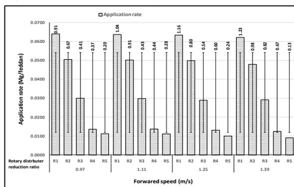
**Fig. 11. Effect of rotary distributor speed at different planting forward speeds on fertilizer application rate**
