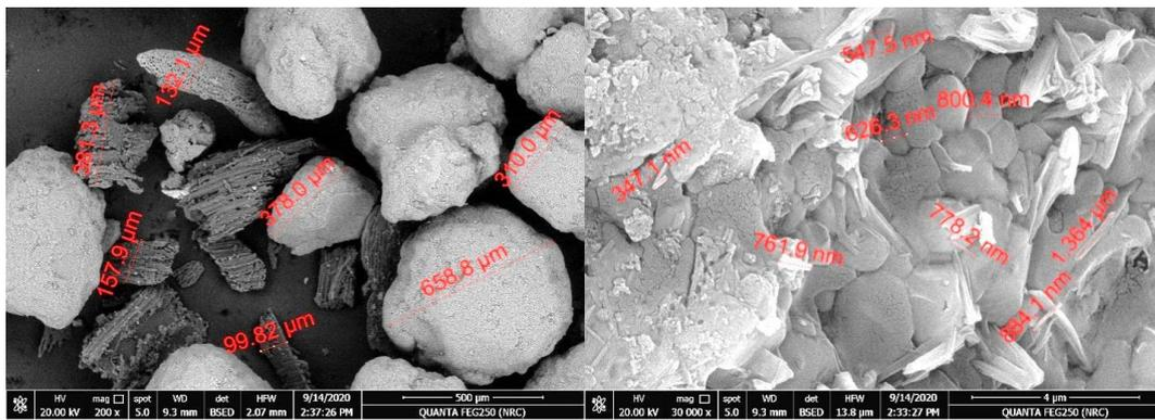
(A). An image of the maximum granules size under the electronic microscope (Scale 1: 200)
