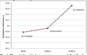
Fig. 6. The relationship between pressure and distribution uniformity
