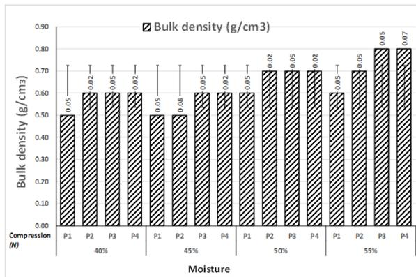
a) Effect of pressure value and moisture content on bulk density
