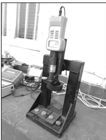
**Fig. 3.** An image for the manual briquetting device
