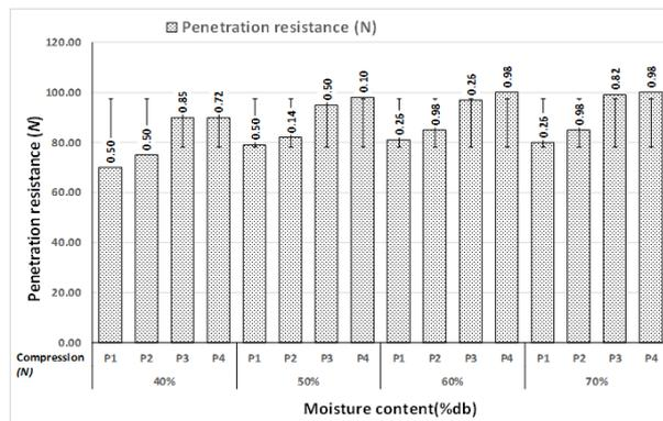
**b) Effect of pressure and moisture content on penetration resistance**
