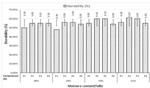
d) Effect of pressure value and moisture content on durability
