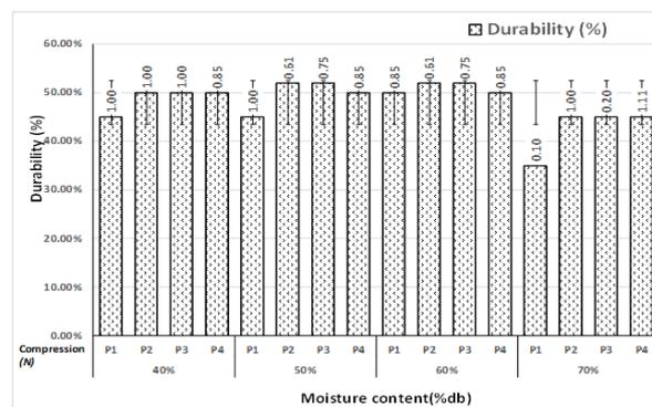
**d) Effect of pressure value and moisture content on durability**
