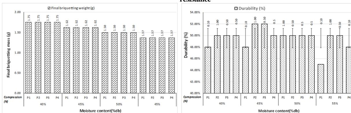
**c) Effect of moisture content on final briquette mass      d) Effect of pressure value and moisture content on durability**
