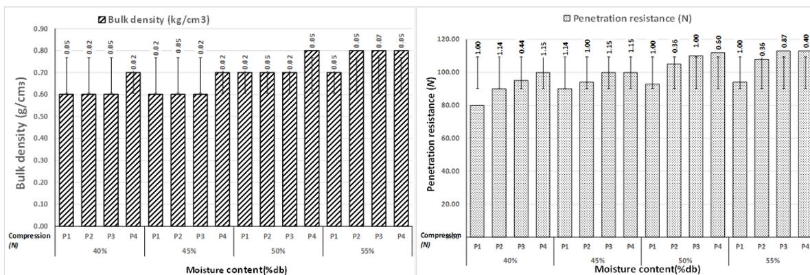
**a) Effect of pressure value and moisture content on bulk density      b) Effect of pressure and moisture content on penetration resistance**
