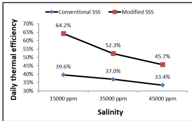
Fig. 7. Daily thermal efficiency of both conventional and modified SSSs at different salinity levels.
