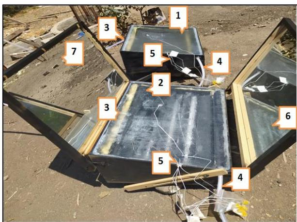
1- Conventional SSS without mirrors 2- Modified SSS with booster mirrors 3-Inlet of saline water 4- Outlet of distillate water 5-Thermocouples 6-Bottom booster mirror 7-Top booster mirror
