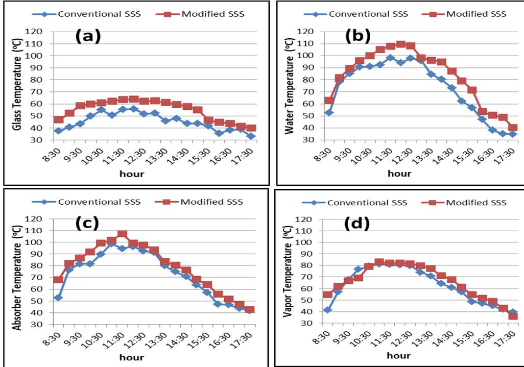
Fig. 4. Variations of average hourly temperatures of: (a) glass, (b) water, (c) absorber and (d) vapor, for both conventional and modified SSSs.
