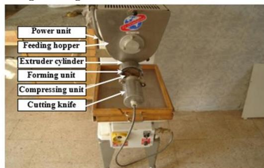
**Fig.1. Extruder pelleting machine**
