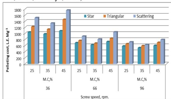
Fig. 9. Influence of extruder screw speed on the cost of pelleting process at different moisture content and holes distribution on the die surface.
