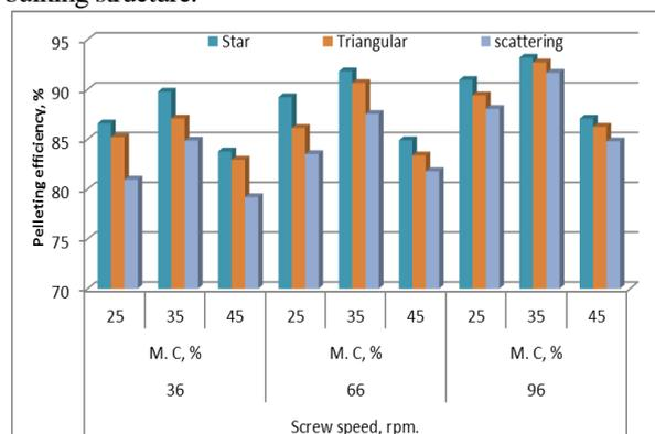
Fig. 4. Influence of extruder screw speed on pelleting effectiveness at various moisture content and holes distribution on the die surface.
