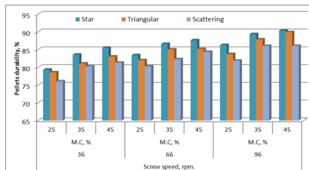
**Fig. 6. Influence of extruder screw speed on pellets durability at various moisture content and holes distribution on the die surface.**
