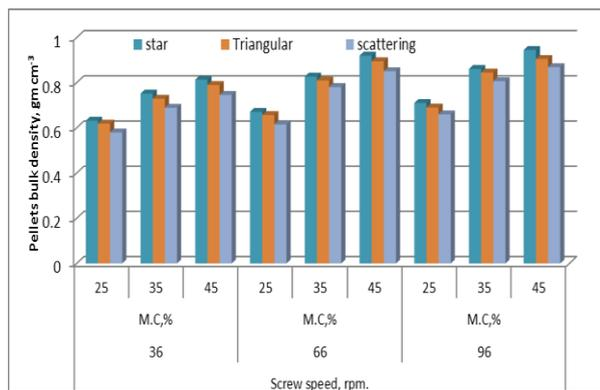
**Fig. 5. Influence of extruder screw speed on pellets bulk density at various moisture content and holes distribution on the die surface.**
