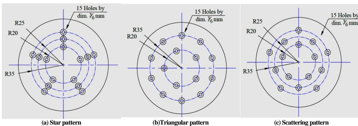
**Fig. 2. Different patterns/shapes of surface holes distribution of extruder die**
