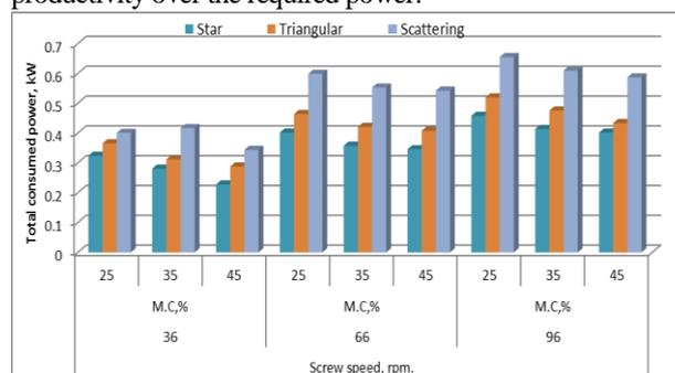
**Fig. 7. Effect of extruder screw speed on total consumed power at different moisture content and holes distribution on the die surface.**
