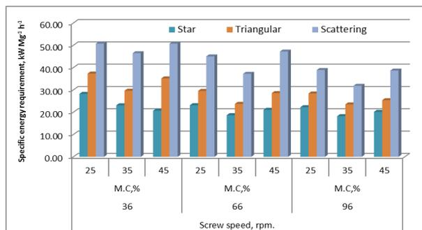
Fig. 8. Effect of extruder screw speed on specific energy requirement at different moisture content and holes distribution on the die surface.
