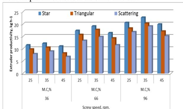
Fig. 3. Influence of extruder screw speed on productivity at various moisture content and holes distribution on the die surface.
