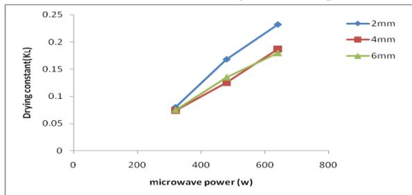
Figure 5. Relationship between (p) and “KL” at different (Th)
