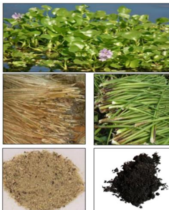
Figure 1. Water hyacinth preparation for pyrolysis and the resulting biochar.
