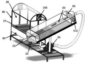
Fig. 1. A schematic for the tested hybrid solar dryer with auxiliary heaters.
