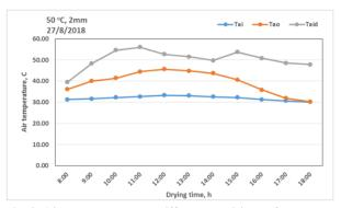
Fig.3. Air temperature at different positions of the dryer as related to drying time at drying air temperature (50 °C).
