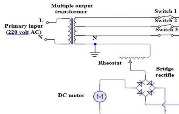
**Fig. 4. Power circuit of metering device.**
