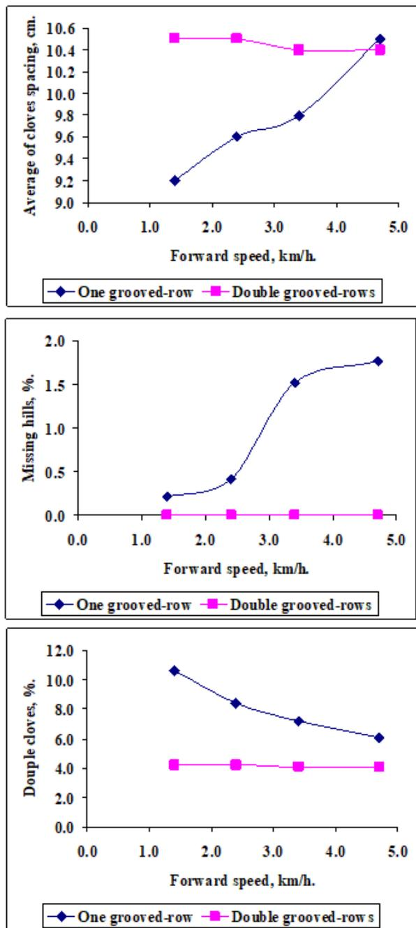
**Fig.14. Effect of planter forward-speed on average garlic-cloves spacing and missing hills percent using one and double grooved-rows.**
