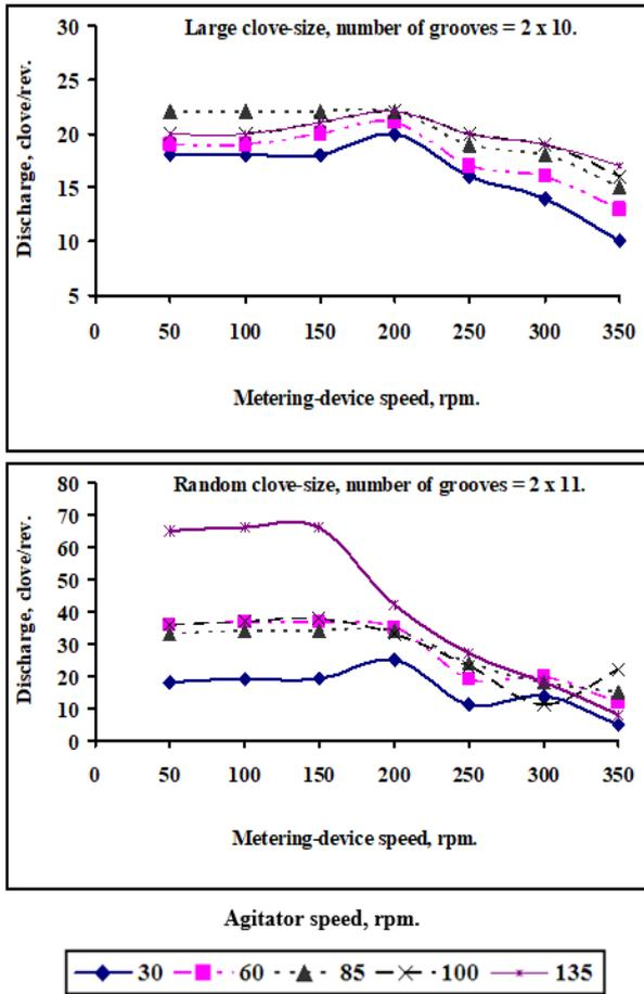
Fig. 8. Effect of metering-device and agitator speeds on garlic-cloves discharge for large and random clove-sizes.
