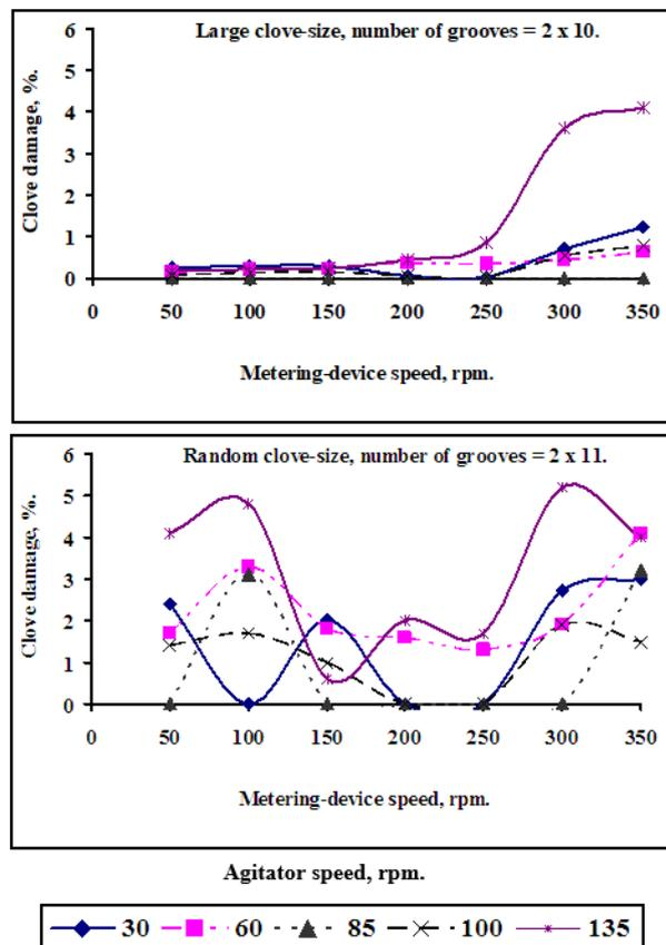
**Fig. 11. Effect of metering-device and agitator speeds on garlic-cloves damage percent for large and random clove-sizes.**
