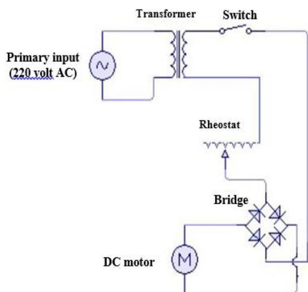
Fig. 5. Power circuit of agitator.
