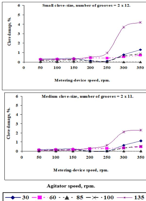
**Fig. 10. Effect of metering-device and agitator speeds on garlic-cloves damage percent for small and medium clove-sizes.**
