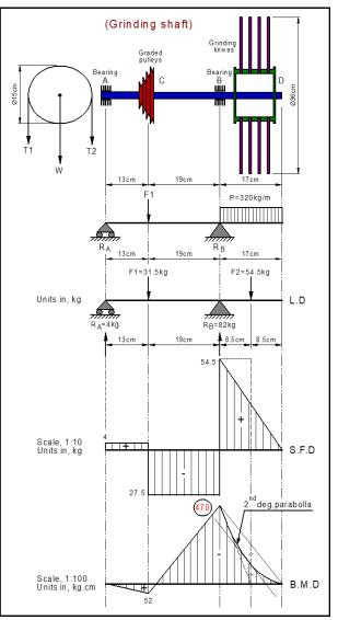
Fig. 3. Stress analysis on grinding shaft.
