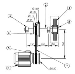
Fig. 2. Power transmission from electric motor to grinding shaft.
