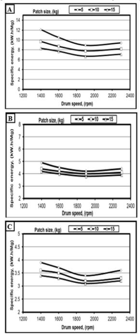
Fig. 6. Effect of drum speed on specific energy at different patch sizes and different screen diameters.
