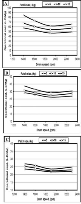
Fig. 7. Effect of drum speed on operational cost at different patch sizes and different screen diameters.
