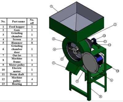
Fig.1. 3D drawing of the developed grinding machine.
