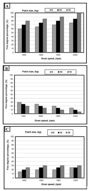
Fig. 5. Effect of drum speed on machine fines degree at different patch sizes and different screen diameters.
