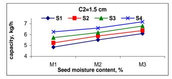
Fig (5-3) Effect of disc-housing clearance on separating capacity
