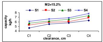
Fig (5-2) Effect of disc-housing clearance on separating capacity
