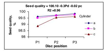
Fig (2-A) Effect of spikes position on disc and cylinder on seed quality
