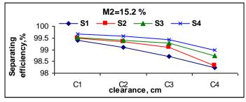
Fig (4-2) Effect of clearance on separating efficiency
