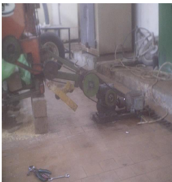
Fig. (3): Developed setup using electric motor and reducing speed unit to drive the ground wheel shaft during laboratory test of seed drill.
