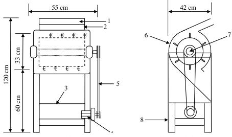
1 - Input , 2- Feed hopper, 3 – Output, 4 – Power unit, 5 - V. belt, 6 – Housing, 7 - Drum shaft, 8- Frame
