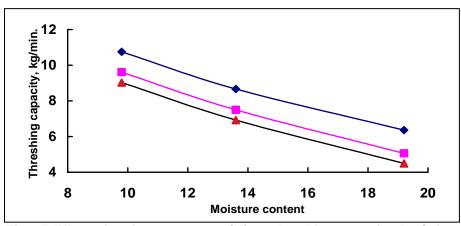
Fig. 15 Effect of moisture contents(M) on threshing capacity, kg /min.at different levels of spikes number and position (P).
