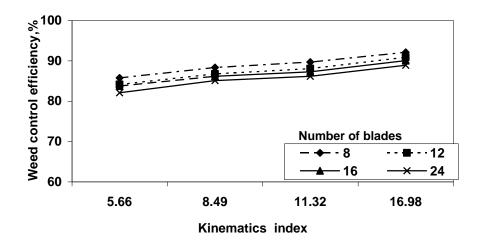
Fig. (3): Effect of kinematics index and the number of cultivator blades on the weed control efficiency at an angle of 90°.
