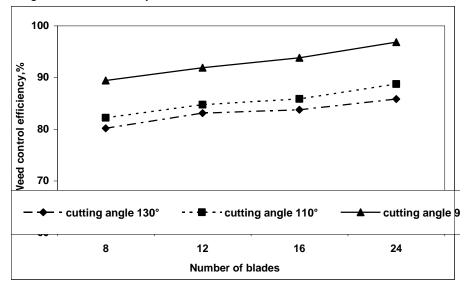
Fig. (2): Effect of the cutting angle and the number of cultivator blades on weed control efficiency.
