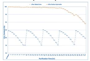
Fig. 10. Methane content in biogas after the purification process using mechanical stirring method at speed of 200 rpm.
