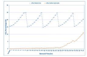
Fig. 9. Carbon dioxide percentage in biogas after purification process using mechanical stirring method at speed of 200 rpm.
