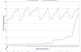
Fig. 5. Carbon dioxide percentage in biogas after purification process using manual stirring method.
