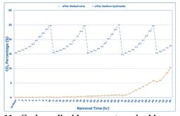
Fig. 11. Carbon dioxide percentage in biogas after purification process using mechanical stirring method at speed of 150 rpm.
