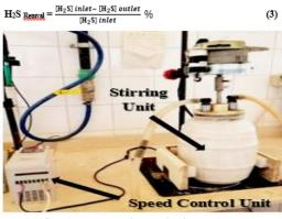
Fig. 1. Mechanical stirring system.
