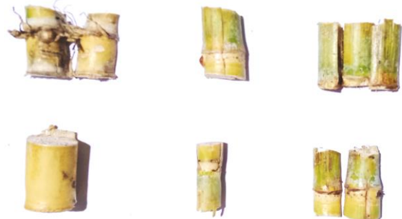
Figure 15. Different types of nodes damage during machine testing.
