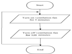
Fig. 6. Flow chart for the ventilation control subroutine.
