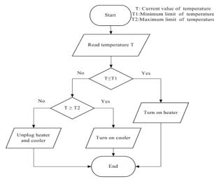
Fig. 4. Flow chart for the temperature control subroutine.
