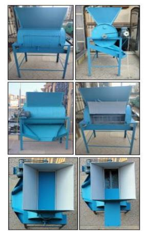
Fig. 1. Some photos of the developed maize shelling machine.
