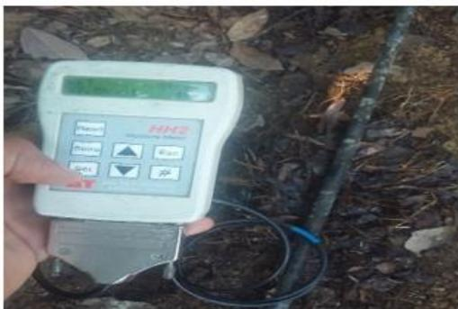
Figure 3. Moisture meter instrument type (HH2)
