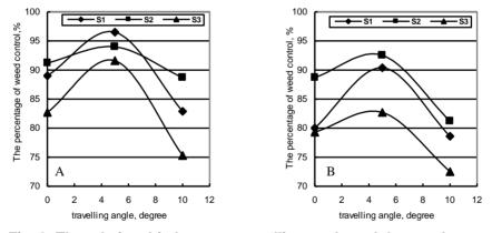
Fig. 2: The relationship between travelling angle and the weeds control A- after cultivation directly B- 5 days later after cultivation
