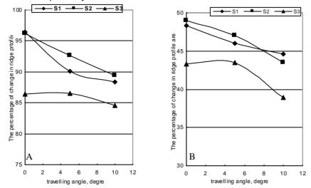
Fig. 6: The relationship between travelling angle and the percentage of change in ridge profile A-after the first cultivation B- after the second cultivation
