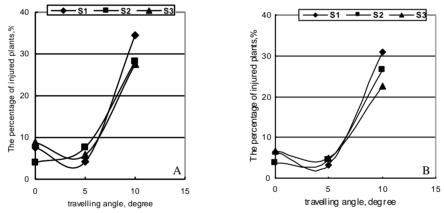
Fig. 4: The relationship between travelling angle and injured plants. A- directly after cultivation B- 5 days later after cultivation
