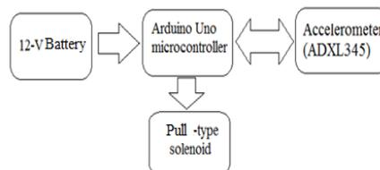
**Fig. 2. Flow chart of the electronic circuit**
