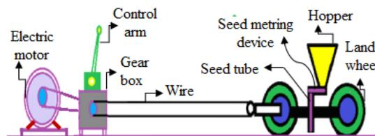
**Fig. 5. Sketch drawing of the developed seed metering device calibration**
