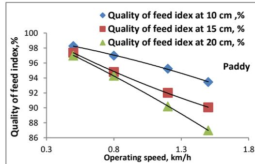
Fig. 8. Effect of the operating speed and distance between hills on Quality of feed index.
