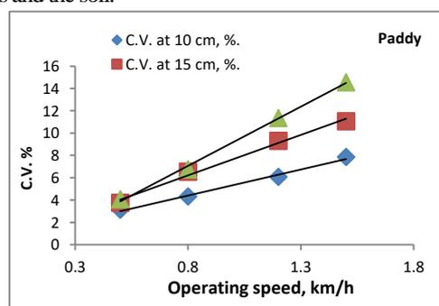
Fig. 9. Effect of the operating speed and distance between hills on seeds longitudinal deviation
