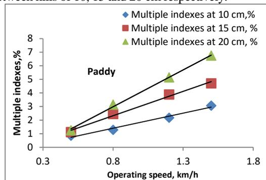
Fig. 7. Effect of the operating speed and distances between hills on multiple indexes
