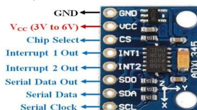
**Fig. 4. The accelerometer (ADXL 345)**
