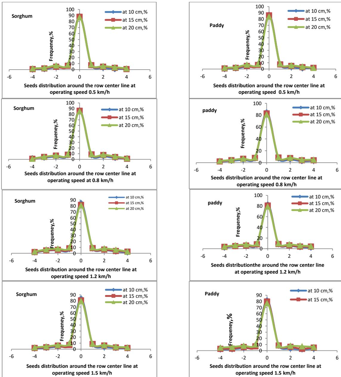
**Fig. 10. Effect of operating speed and distance between hills on the lateral deviation**
