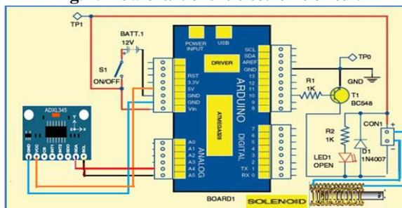
**Fig. 3. Electronic circuit diagram for machine metering device system**
