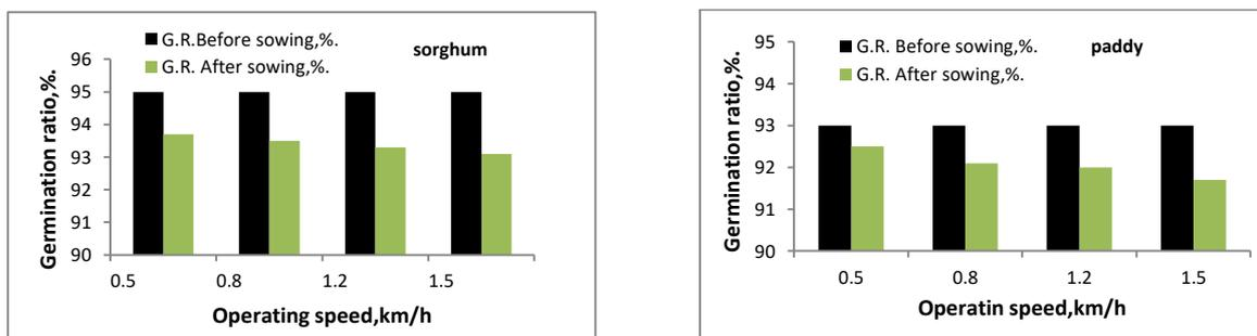
**Fig. 11. Effect of operating speed on the Germination ratio (G.R)**
