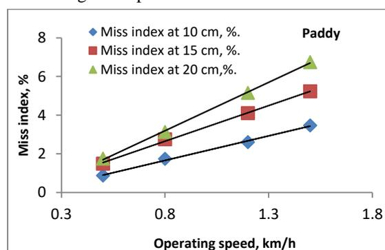
**Fig. 6. Effect of the operating speed and distances between hills on miss index**
