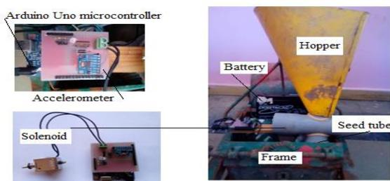
**Fig. 1. Seed metering device mechanism**
