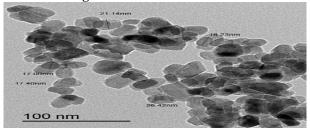
Figure 2. TEM revealed both ZnO NPs small round nanoparticles and big rod nanoparticles.
