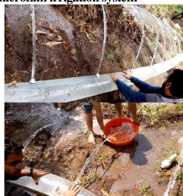
Fig. 3. Measurements of orifices water head and flow rate Pumping unit and its components
