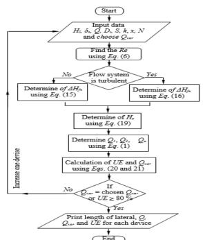
Figure 3. Software model flow-chart for the best length of micro-irrigation laterals using microtube determination.
