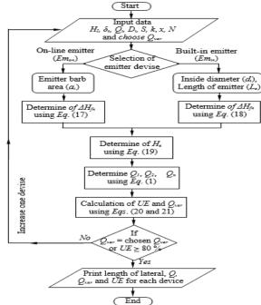
Figure 4. Software model flow-chart for the best length of micro-irrigation laterals using different devices determination.
