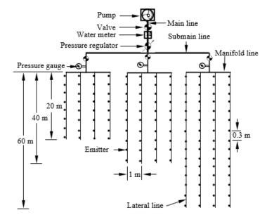
Figure 5. A schematic plan of the tested emitter devices with different lengths of lateral.
