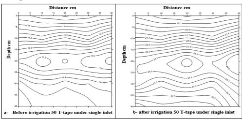
Fig. 8. Soil moisture distribution (a) before and (b) after irrigation under using single inlet with T-tape lateral under lateral length 50 cm.
