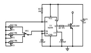
Fig. 1. Ultrasonic generator circuit
